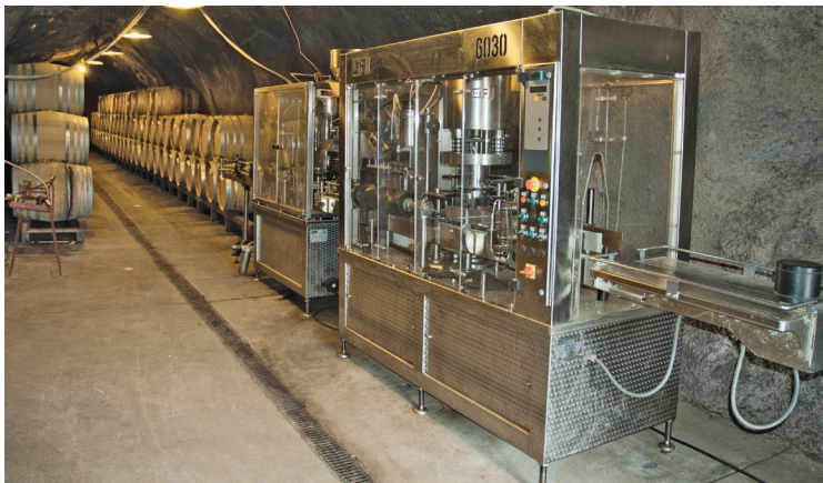
Eight-spout filler/corker monobloc is adjacent to wine tanks on the crush pad at Mount Eden and is used for average 900 cases per day bottling.
